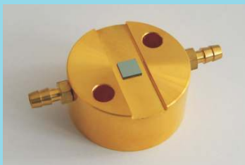
soldered chip on water cooled mount with 25.0mm diameter
